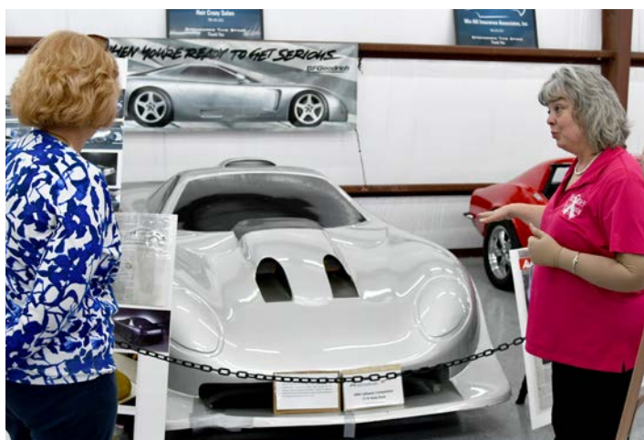
Board member Phyllis Weller shows a visitor the 1994 Callaway competition "body buck." The buck is a pattern. Reverse molds are made from the buck and used to produce body parts for the actual racecar.
